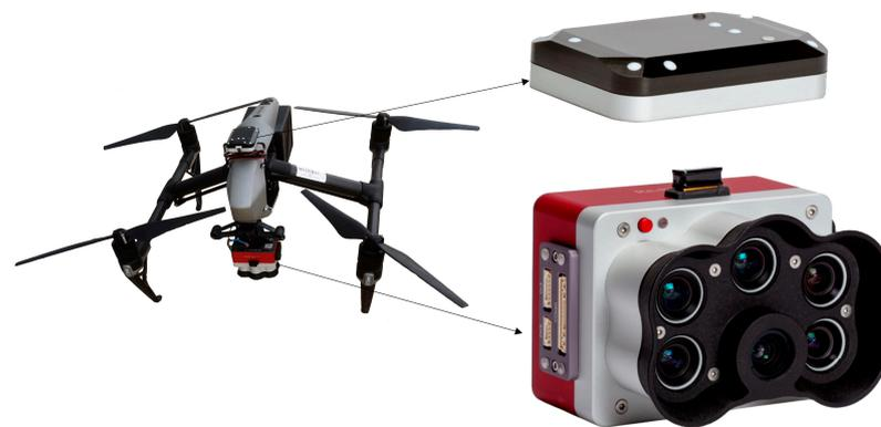
Figure 2. Unmanned aerial vehicle multispectral image acquisition system.
