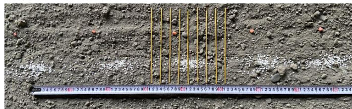
Figure 10. The fertilizer distribution when the operating speed was 3 \text{ km}\cdot\text{h}^{-1} and the seed spacing was set to 20 cm.
