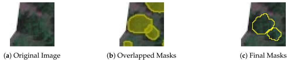
Figure 19. Resolving overlapped masks. (a) Original image. (b) Overlapped masks from Detectron2. (c) Separated masks from the proposed method.
