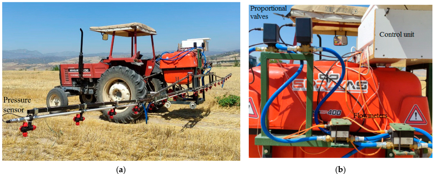
Figure 1. Sprayer system with application rate controller. (a) Boom sections and pressure sensors; (b) proportional valve and flow meter connection.
