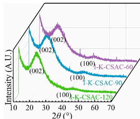
**Figure 18.** XRD patterns of I-K-CSAC-60, I-K-CSAC-90, and I-K-CSAC-120.
