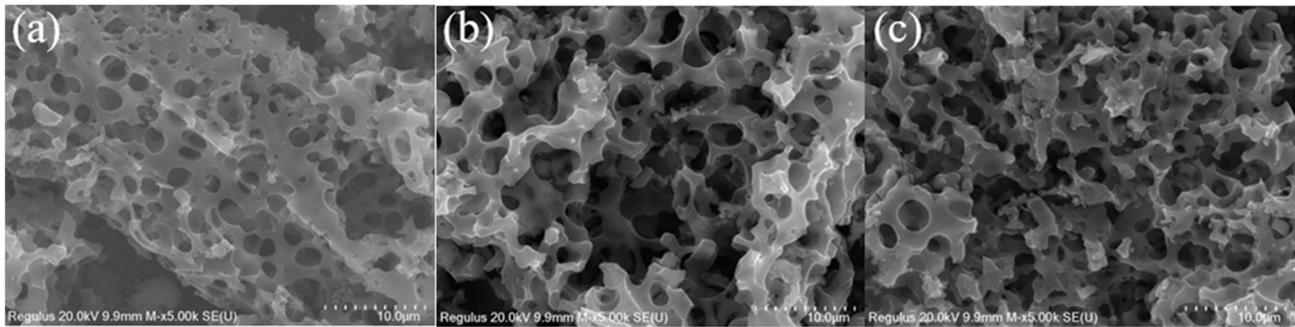
**Figure 11.** SEM images of (a) I-K-CSAC-600, (b) I-K-CSAC-700, and (c) I-K-CSAC-800.
