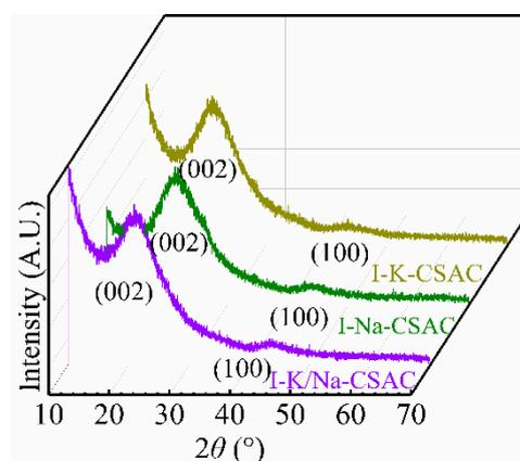
**Figure 14.** XRD patterns of I-K-CSAC, I-Na-CSAC, and I-K/Na-CSAC.
