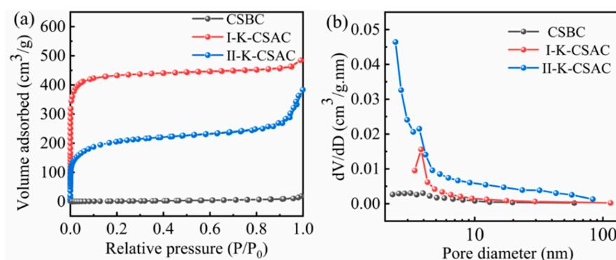
**Figure 7.**  $N_2$  adsorption/desorption isotherms (a) and pore size distributions (b) of CSBC, I-K-CSAC and II-K-CSAC.
