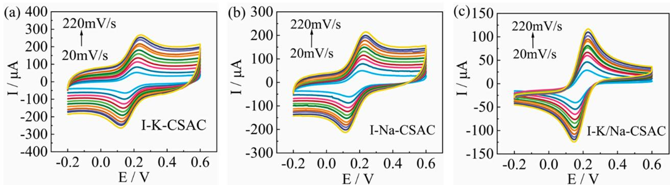
**Figure 16.** CV curves of (a) I-K-CSAC, (b) I-Na-CSAC, and (c) I-K/Na-CSAC.
