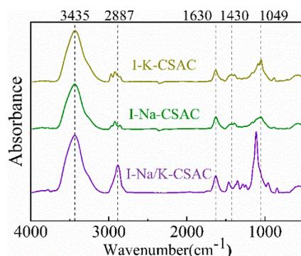
**Figure 13.** FTIR spectra of I-K-CSAC, I-Na-CSAC, and I-K/Na-CSAC.
