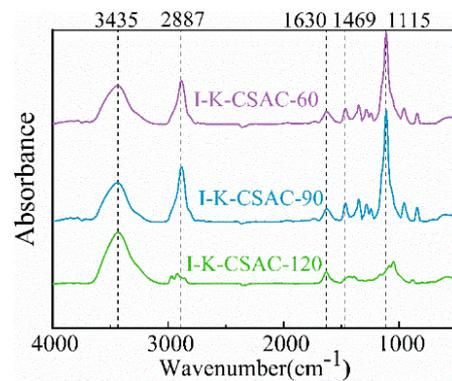
**Figure 17.** FTIR spectra of I-K-CSAC-60, I-K-CSAC-90, and I-K-CSAC-120.
