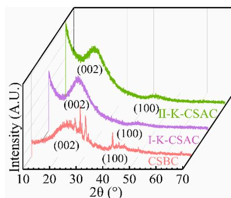
**Figure 5.** XRD patterns of CSBC, I-K-CSAC, and II-K-CSAC.
