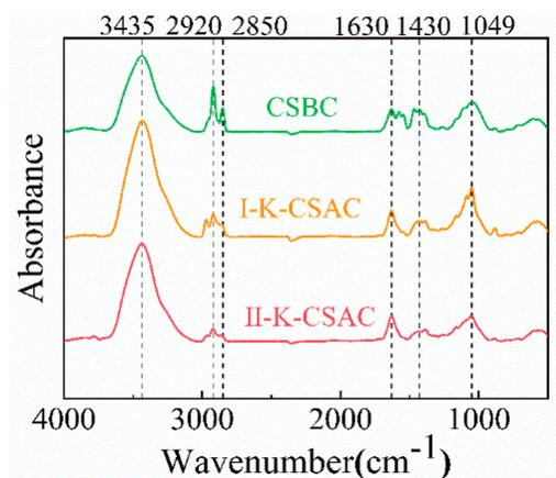
**Figure 4.** FTIR spectra of CSBC, I-K-CSAC, and II-K-CSAC.
