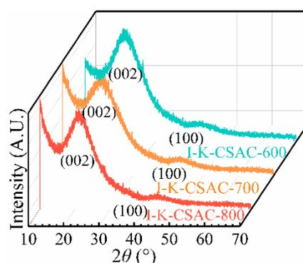
**Figure 10.** XRD patterns of I-CSAC-600, I-CSAC-700, and I-CSAC-800.
