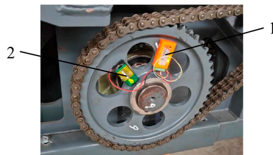
Figure 3. Experimental setup for torque measurement: 1. TQ201 wireless torque sensor node and 2. battery.
