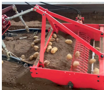
Figure 15. Potato pile up and roll back Situation.
