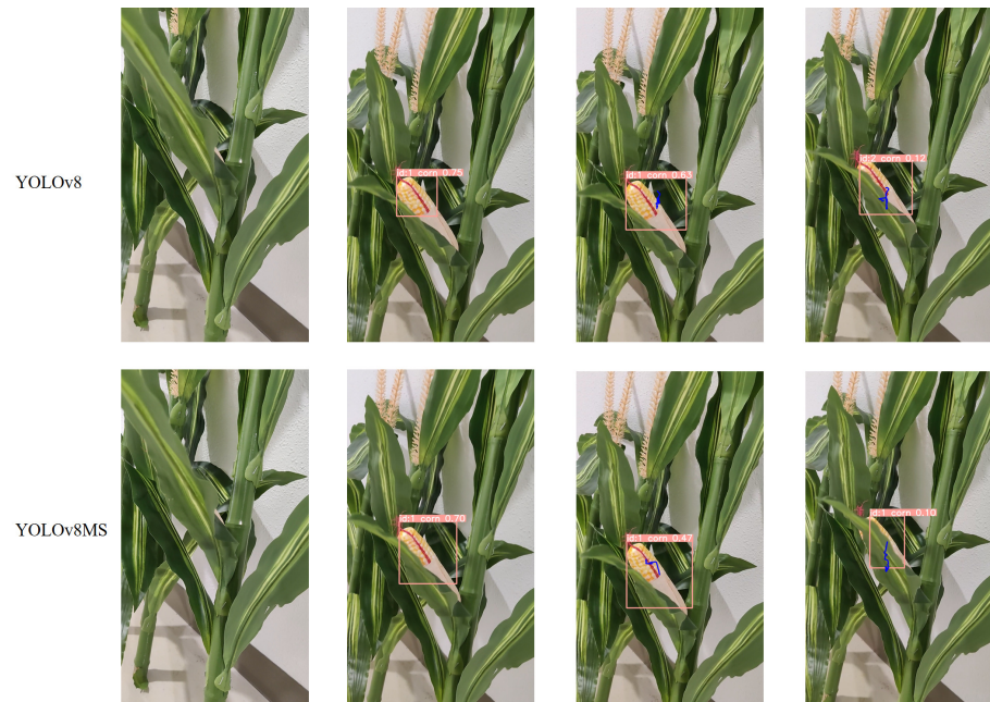
Figure 10. The image shows frames grabbed from the video, demonstrating that YOLOv8MS can detect corn more accurately under occlusion. The blue line represents the corn tracking trajectory.
