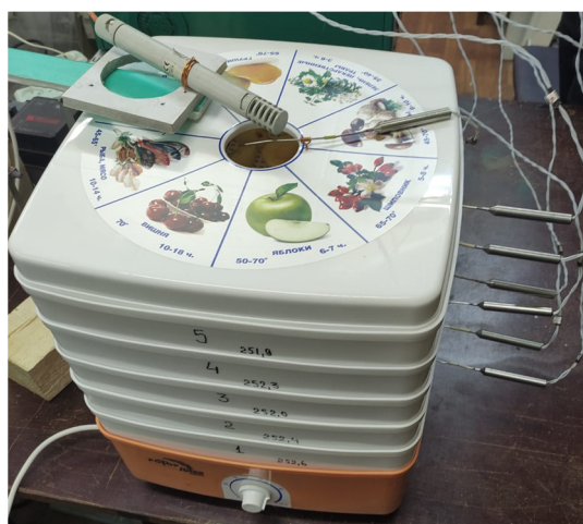
Figure 4. Overall view of the convective-type dryer ROTOR SH-002 with temperature and humidity sensors.
