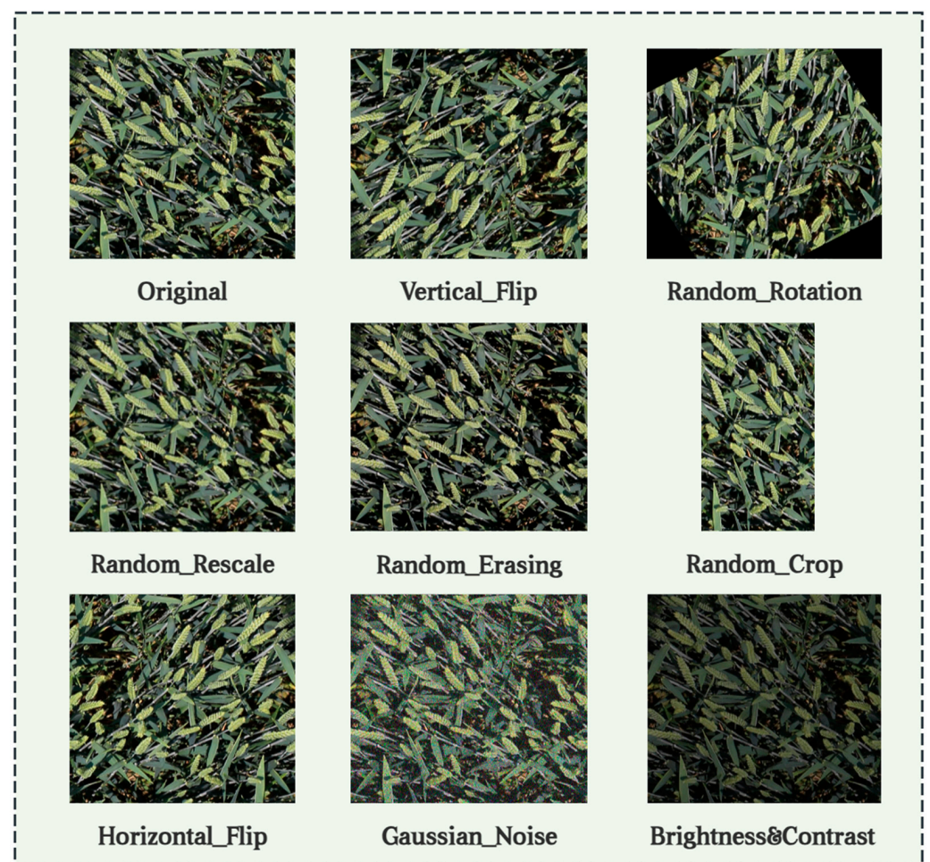
Figure 2. This image illustrates several data augmentation techniques applied to wheat spike images to simulate environmental variations. Techniques include the original, unmodified control; vertical
