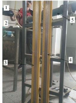
**Figure 3.** Pressure test. Note: 1 denotes the pest vacuum, 2 denotes the air hose, 3 denotes the U-shaped tube for reading static pressure, 4 denotes the U-shaped pipe for reading differential pressure, and 5 denotes the pipe fitted with a Venturi nozzle, which is connected to the export of the pest vacuum.
