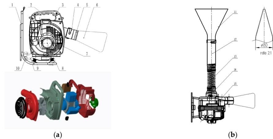
**Figure 1.** The structure of the pest vacuum. Note: 1 back rack, 2 handlebar, 3 flame rollout switch, 4 vent connector, 5 lathe dog, 6 collection bags, 7 housing, 8 gasoline engine, 9 accelerator flexible shaft, 10 accelerator switch, 11 suction port, 12 suction pipe, 13 flexible suction pipe, 14 connection pipe, 15 top cover. (a): Front view; and (b): vertical view.
