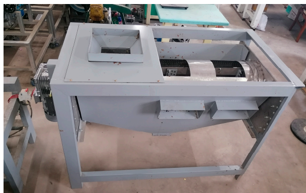
Figure 13. Seed melon crushing and seed-extraction separator and test process.
