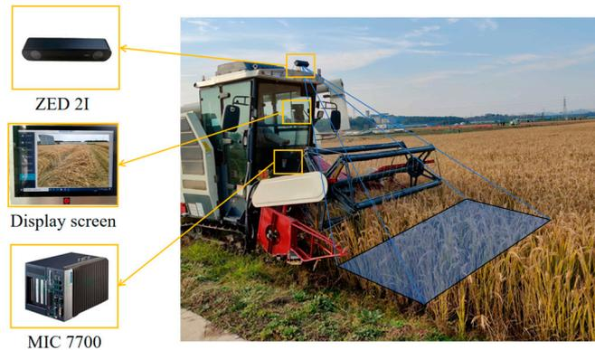
**Figure 1.** Visual data acquisition system for feed quantity.
