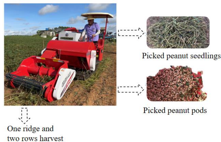
Figure 13. Field test of fresh-peanut-picking crawler combine harvester.
