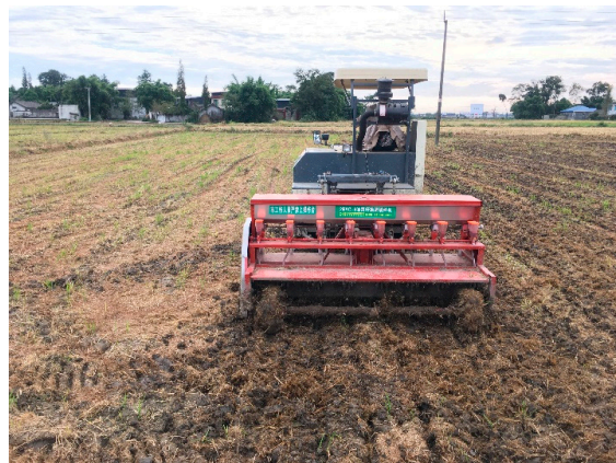
Figure 2. Field operation of the strip-tillage oilseed rape seeder.
