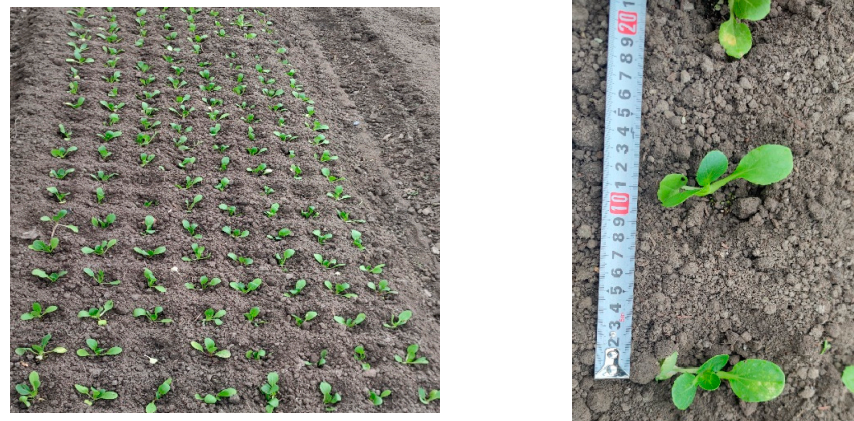
Figure 19. Planting mechanism performance test: (a) test effect; and (b) measurement of plant spacing.
