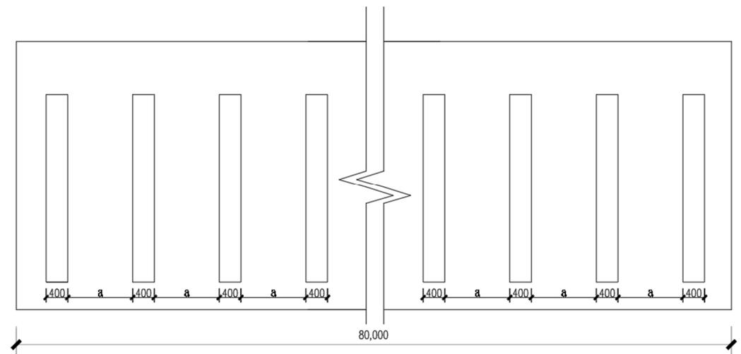
**Figure 3.** The top-view design of the double-slope greenhouse shade room roof windows.
