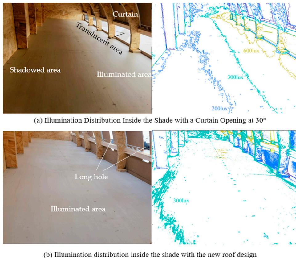
**Figure 16.** Illumination distribution inside the shade rooms with different roof types.
