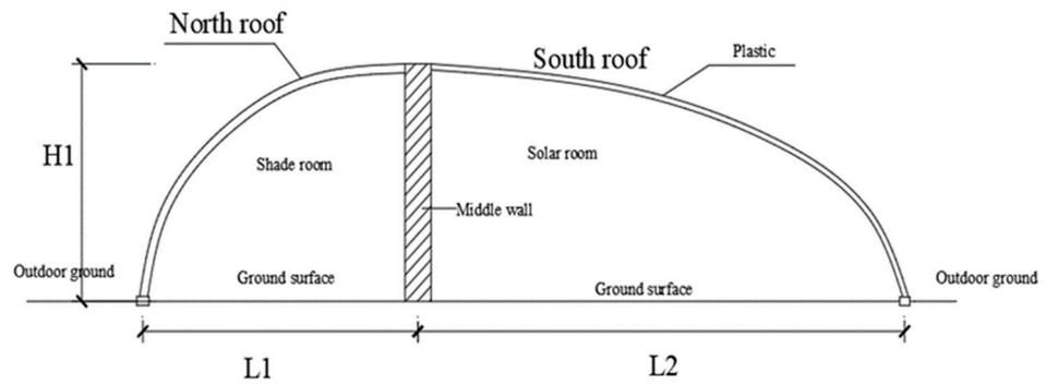
Figure 1. Section of double-slope greenhouse.
