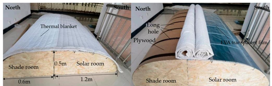
**Figure 4.** Double-slope greenhouse: equal-scale 1:8 model.
