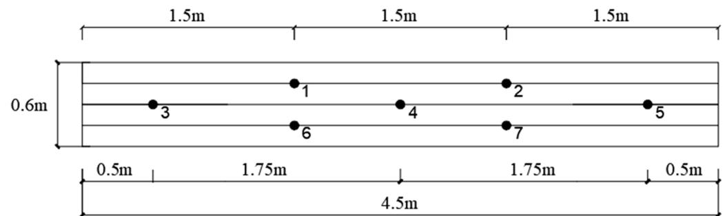
**Figure 6.** Arrangement of light sensor points in the shade room.
