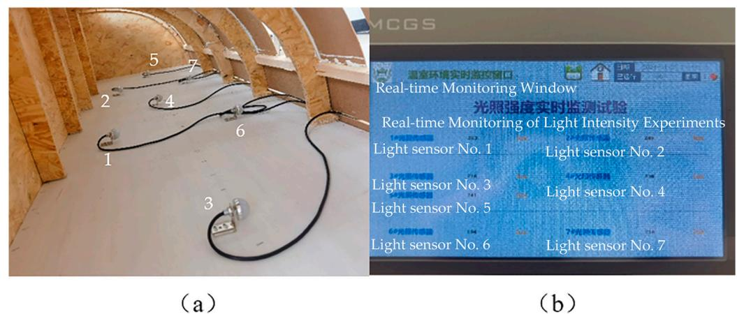
**Figure 7.** (a) Actual arrangement of light level sensors in the shade room. (b) Light intensity monitoring interface.
