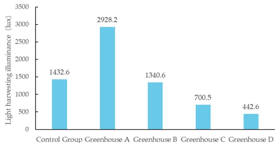
**Figure 12.** Five double-slope greenhouse shade room light illuminance histograms.
