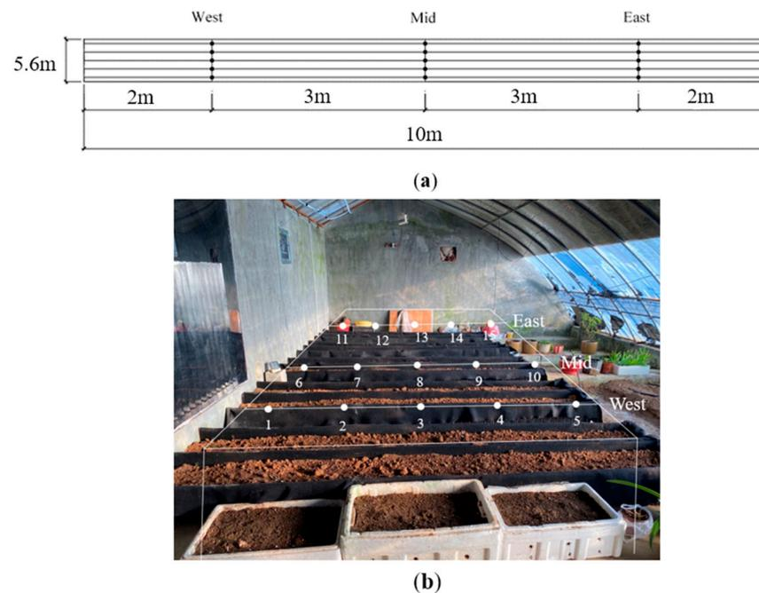
**Figure 5.** (a) Layout of solar radiation measurement points in the greenhouse. (b) Layout of solar radiation measurement points in the field.
