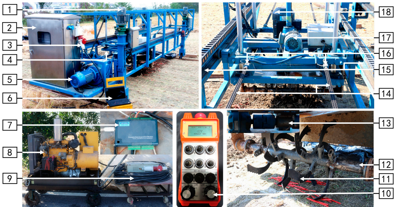
Figure 3. Overview of the in situ test rig: 1. Column lifting motor, 2. Control system, 3. Power connection interface, 4. Carriage unit, 5. Pulling motor, 6. Data collection computer, 7. Data collection unit, 8. Diesel-driven generator, 9. Power transmission cable, 10. Operating handle, 11. Rotary blade, 12. Driving shaft, 13. Torque sensor, 14. Drawing chain, 15. Guide rail, 16. Force sensor, 17. Power screw and motor, 18. Rotary motor.
