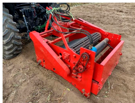
Figure 13. Field experiment of potato drip irrigation tape recycling machine.
