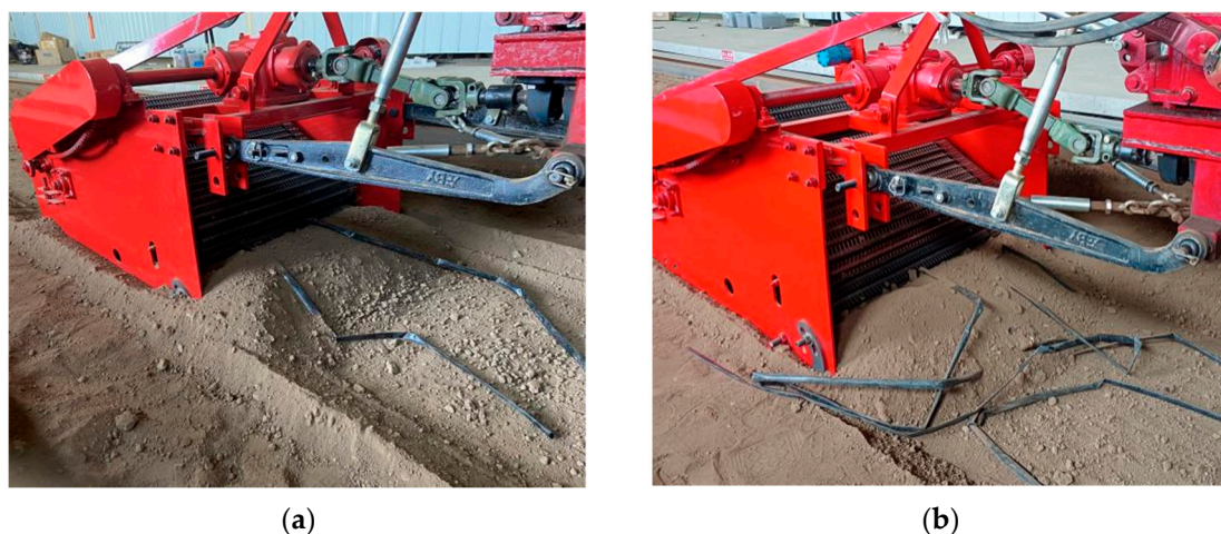
Figure 15. Single-Factor experiment process. (a) Recycling status at lower machine forward speed; (b) Accumulation phenomenon of drip irrigation tape.
