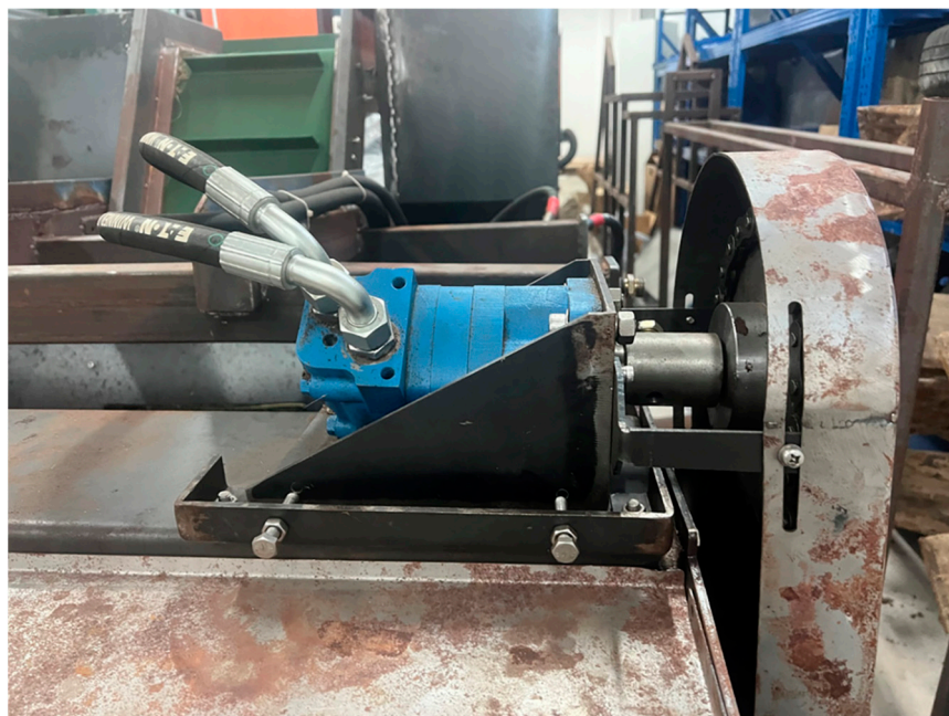
Figure 13. Installation diagram of the tine drum hydraulic motor.
