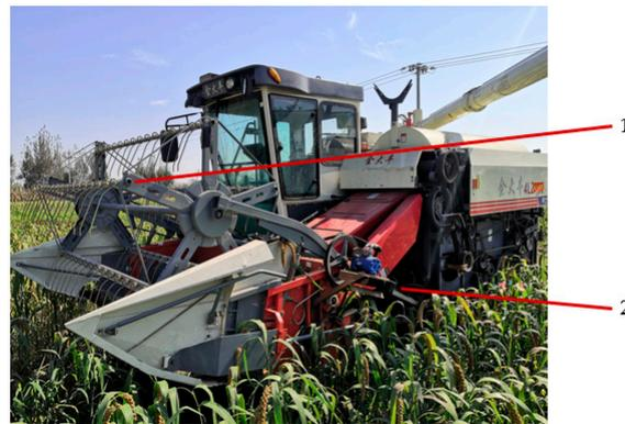
**Figure 12.** 4LZ-6B Millet combine harvester. 1. Reel. 2. Hydraulic motor.
