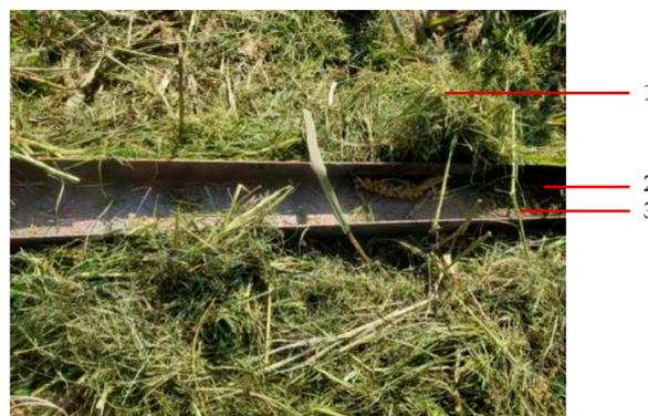
**Figure 13.** Sample trough after harvesting. 1. Stems. 2. Sampling trough. 3. Grains header loss.
