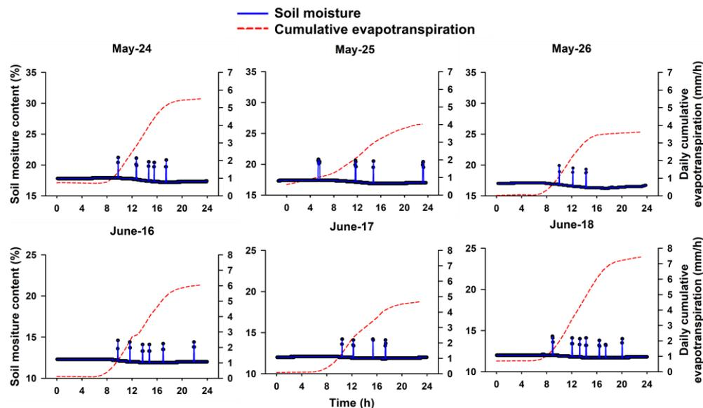
Figure 4. Soil moisture content and daily cumulative evapotranspiration from 24 to 26 May and from 16 to 18 June. Soil moisture content was measured using a soil moisture sensor in 100%  $ET_c$  measured by the KMA (Korea Meteorological Administration), and cumulative evapotranspiration was measured based on the KMA.
