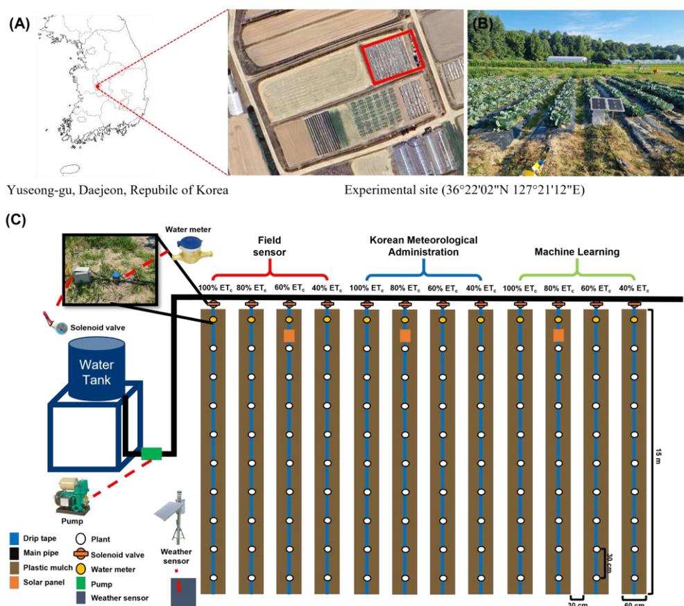
**Figure 2.** Location and layout of cabbage irrigation experiment. (A) Location of experimental site for field cabbage irrigation experiment. (B) 72 days after transplanting. (C) Schematic diagram of the experimental field setup for cultivating cabbages.
