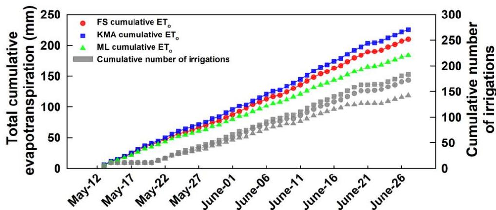
Figure 5. Total cumulative evapotranspiration and number of irrigations of the FS (field sensor), the KMA (Korea Meteorological Administration), and the ML (machine learning) over 46 days (13 May–27 June).
