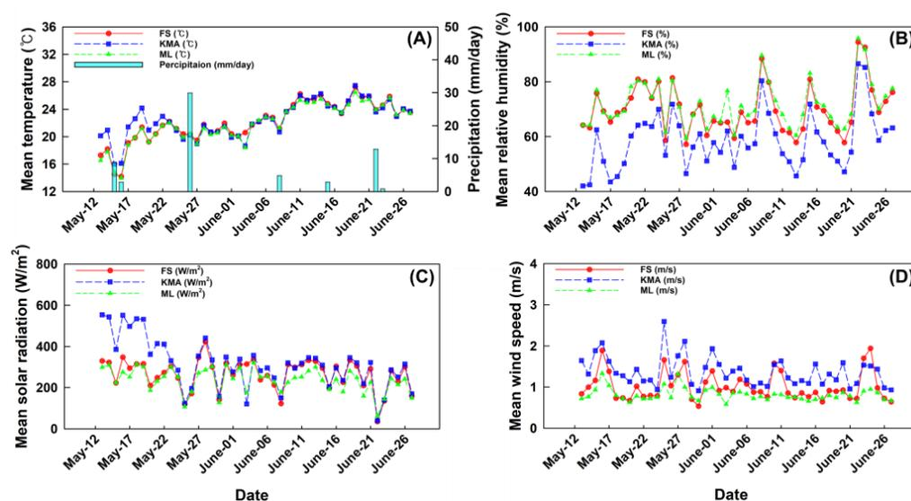
**Figure 3.** Precipitation and daily temperature from 13 May to 27 June. (A) Mean temperature and precipitation, (B) mean relative humidity, (C) mean solar radiation, and (D) mean wind speed were measured by the FS (field sensor), the KMA (Korea Meteorological Administration), and the ML (machine learning). Precipitation was measured by the KMA.
