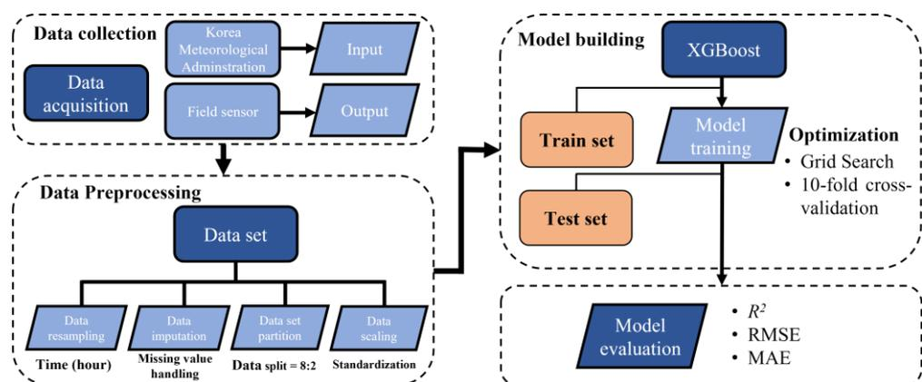
**Figure 1.** Flowchart representing the process of training a virtual sensor based on machine learning (XGBoost Model).
