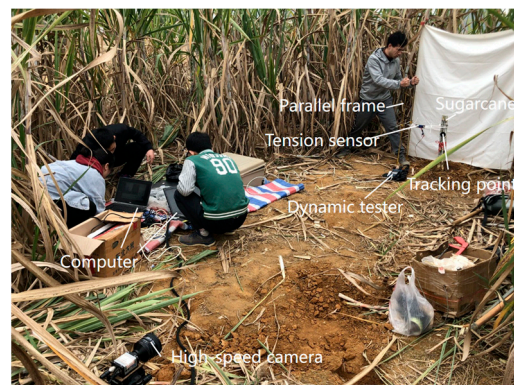
Figure 5. The site of the pull-down test for ratoon sugarcane.
