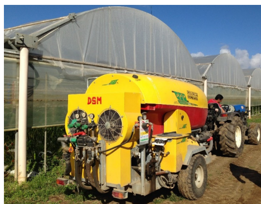
Figure 2. The first spraying system 'Special Serre 2000' used in experimental trials on a protected pepper crop.
