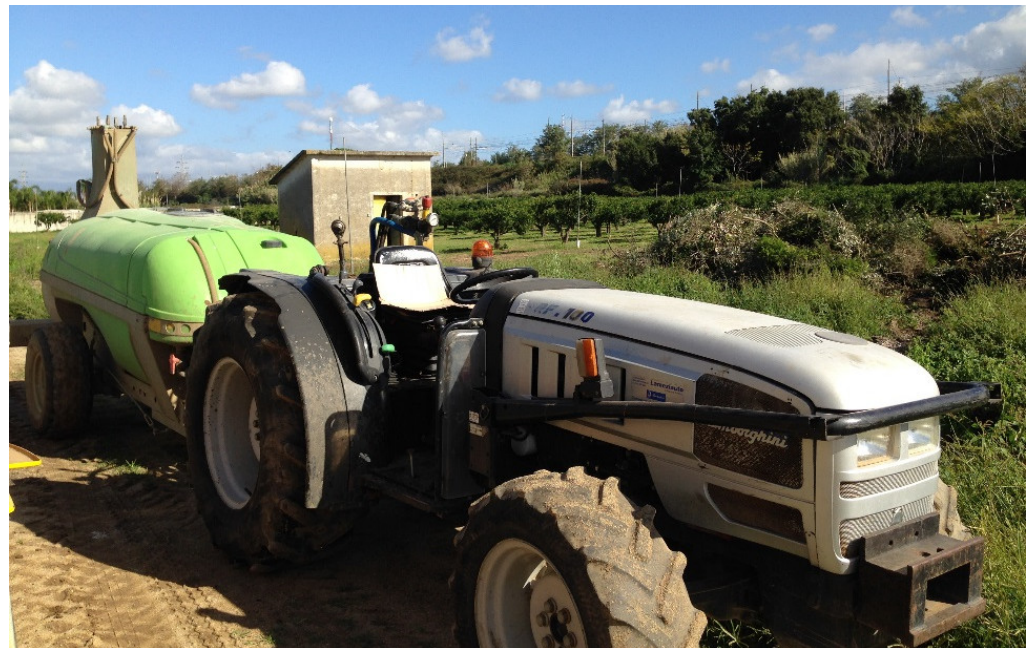
Figure 3. The second spraying system ‘Tifone Storm 2000 80S model’ used in experimental trials on a protected pepper crop.
