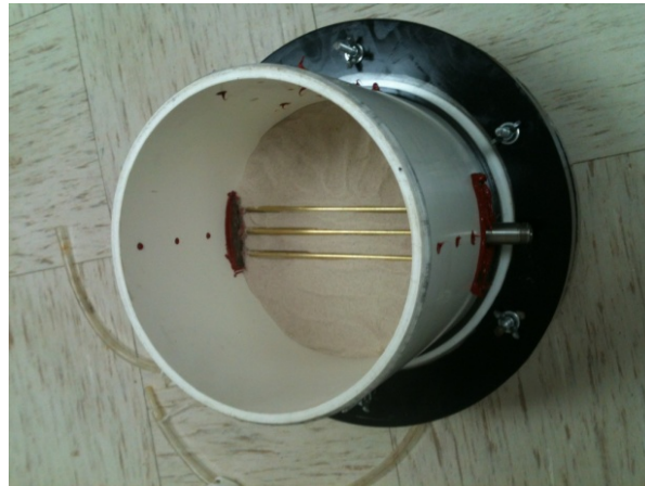
Figure 3. This picture shows the high signal-integrity soil probe flush mounted inside the PVC test column.
