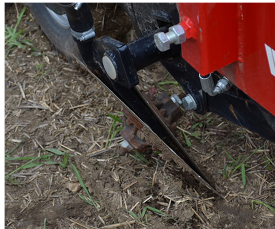
Figure 4. Double-disc opener, in this case not only inclined to the direction of travel, but vertically as well. This provides better seed coverage and less surface soil disturbance.
