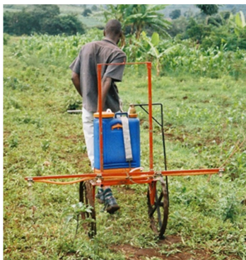
Figure 9. A back-pack sprayer mounted on a wheeled chassis. The sprayer pump is actuated by an eccentric from one of the wheels, the 2-m boom has four nozzles. A manually operated return valve is required to control pressure and prevent wheel skid.
