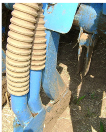
Figure 5. The Turbo Happy Seeder manages rice residue by flailing and lifting it on either side of the chisel-tined no-till slot opener.
