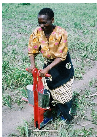
Figure 6. A manually operated jab-planter with hoppers for seed and fertilizer.
