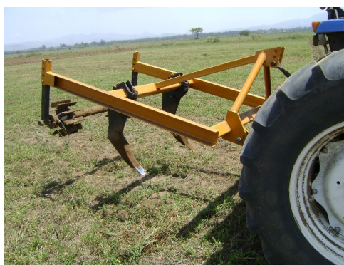
Figure 7. A tractor-mounted chisel-tined ripper which can be used to create narrow tilled strips for crop establishment.
