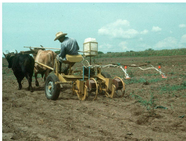
Figure 12. The development of animal-drawn wheeled toolcarriers attracted considerable development effort in the 1980s; however farmer adoption was minimal.
