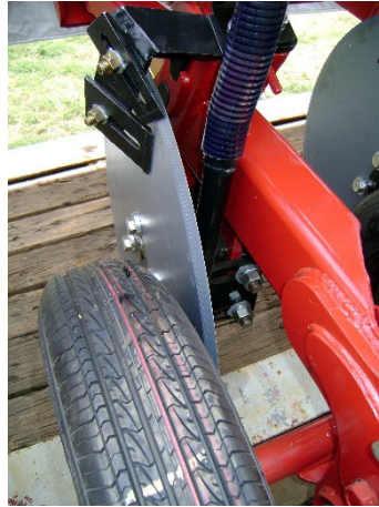
Figure 3. Single inclined disc opener. Seed and fertilizer are delivered behind the disc.
