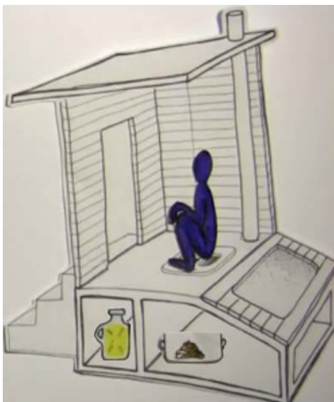
Figure S9: Urine is collected and stored in a urine-diverting dry toilet (UDDT); storage lasts for minimum two months in order to successfully inactivate pathogens (drawing from CaSa-project document, CC).
