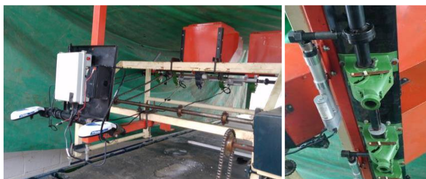
Figure 3. Setup of the test bench with two N-sensors up front connected through the control box with the VRA fertilizer meters (left); close-up view of the fluted rollers connected with the electric actuator piston (right).
