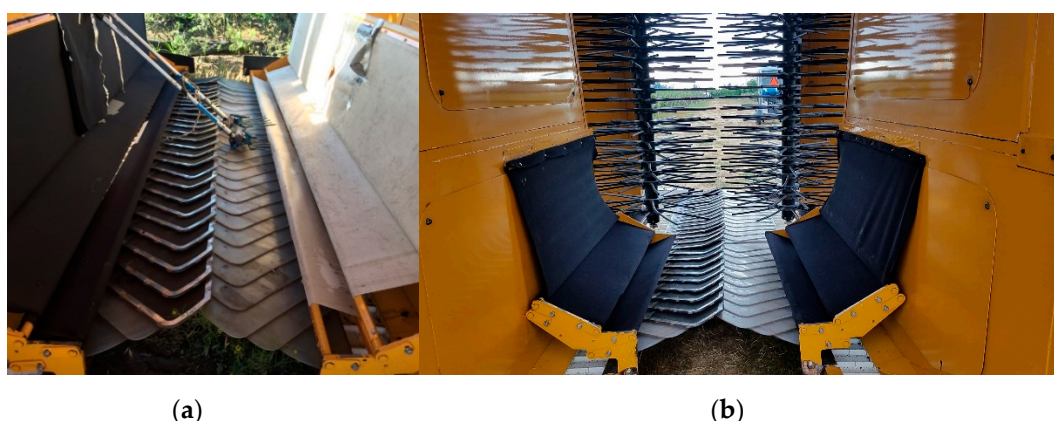
Figure 1. Modifications to an Oxbo 7420 machine harvester for fresh market blueberry. The harvester in Oregon had a neoprene soft catch surface suspended above the conveyor belt and hollowed out catch plates with neoprene installed on the top side of each catch plate (left; a ). A canvas catch surface was installed over the conveyor belt with standard plastic catch plates on the other side of the machine (right; a ). In Washington, both sides of the machine had neoprene catch surfaces, but the catch plates were the same as in Oregon ( b ). Hand held pneumatic shakers were used to harvest ‘Duke’ and ‘Draper’ blueberries in Oregon. ‘Elliott’ and ‘Aurora’ blueberries were harvested with Orbitorator ® picking heads (i.e., rotary drum shakers) in Washington.
