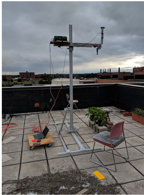
Figure 7. Setup used for data collection. MicaSense RedEdge-3 and ASD FieldSpec are attached on the arm of the rig. Rig was designed to move vertically as well as horizontally to allow for data collection for all three plants at all three heights. Laptop at base of rig was used to run the ASD. Image was taken on 22 September (cloudy day).
