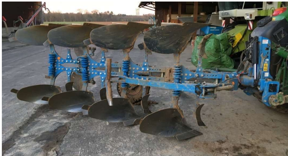
Figure 1. The mounted four-furrow moldboard plow that was used for the tillage operation.
