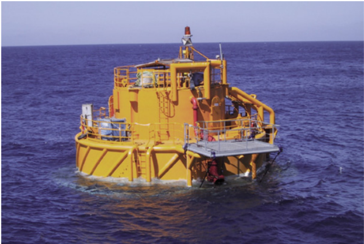
Figure 1. CALM Turret buoy at Apache Stag Field, Australia, Buoy during installation (Reprinted with permission from ref. [49]. Copyright 2011 Bluewater).
