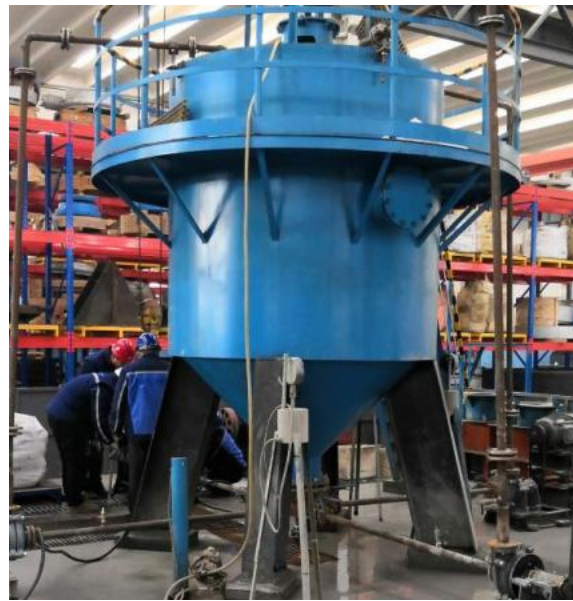
Figure 4. Slurry pump wear test bench.
