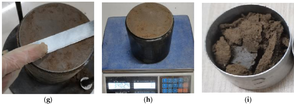
Figure 4. Compaction test of (a) soil sample preparation, (b) net weight weighing of compaction cylinder, (c) placing plastic film on the spacer, (d) assembly of instrument, (e) compaction, (f) layered shaving, (g) topsoil sample troweling, (h) weighing, (i) water content measuring.
