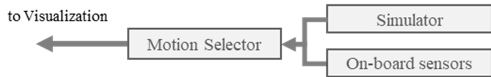
Figure 6. Vessel motion generator module. The operator can choose on-board sensors for real-time motion data or virtual motion for a simulation.
