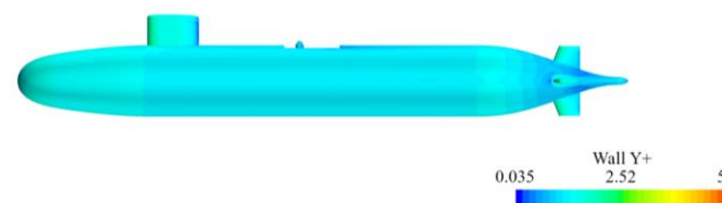
Figure 5. The distribution of Y^+ values on the UUV surface after using the medium grid.
