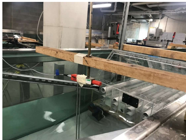
Figure 4. Test model fixed from motion by frames and iron bars as viewed from the back.
