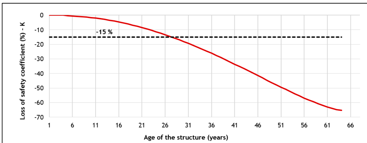
Figure 8. Estimation of the loss of strength capacity over its service life of a structural element working on single flexure with corrosion problems in its main reinforcement.
