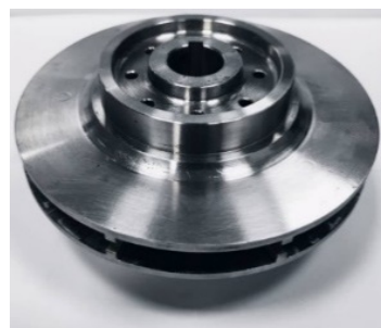
Figure 3. Present TBD pump impeller.
