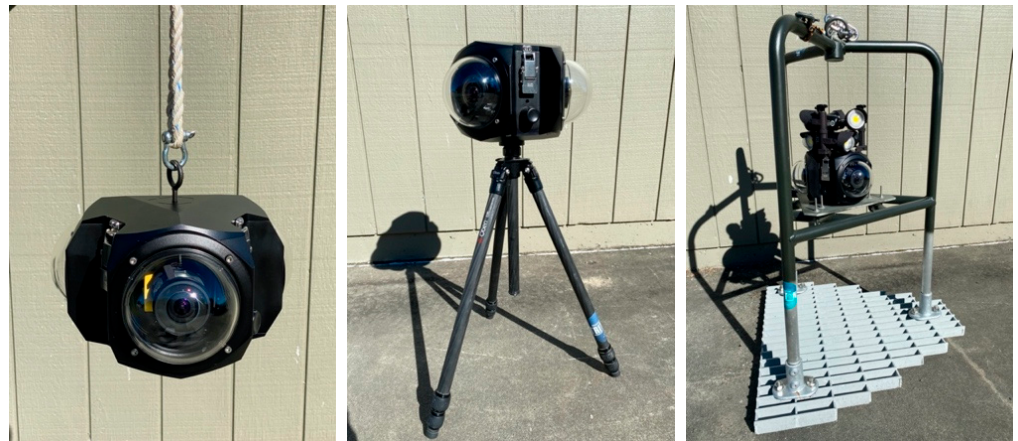
Figure 2. Boxfish in the different configurations: from left to right, hand-held, mounted on tripod, and mounted on lander with external lights on top of the camera.
