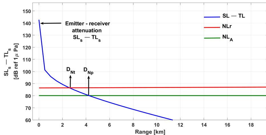
Figure 7. The intersection between the decay curve of the sound level between emitter–receiver and the noise level present in the marine area determines the maximum distance in which SNR = 0. The distances calculated considering the natural ambient noise and natural plus anthropogenic noise will determine the reduction of the communication distance due to marine traffic activity.
