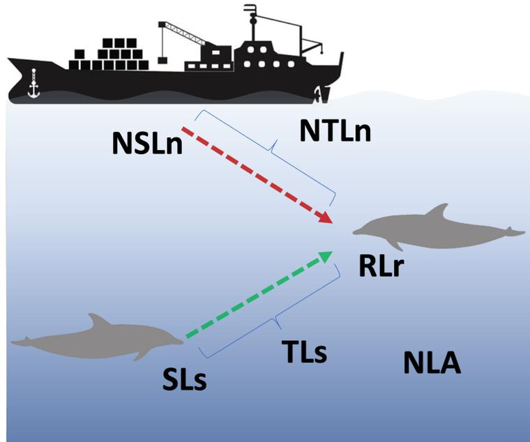
**Figure 5.** Conceptual scheme that represents the communication process between individuals, taking into account all the variables involved in the distance reduction calculation. The variables considered are noise level radiated by the  $n$ -th source  $NSL_n$ , transmission loss calculated from the  $n$ -th source  $NTL_n$ , ambient noise level  $NL_A$ , source level emitted  $SL_s$ , transmission loss from the emitter or source to the receiver  $TL_s$ , and received signal level  $RL_r$ .
