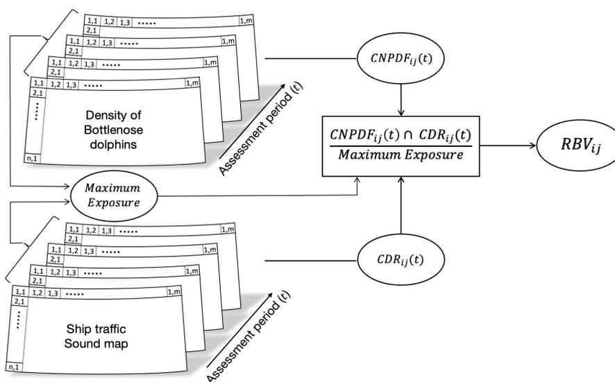
**Figure 9.** Diagram block that summarizes the methodology applied to obtain the risk-based variable.
