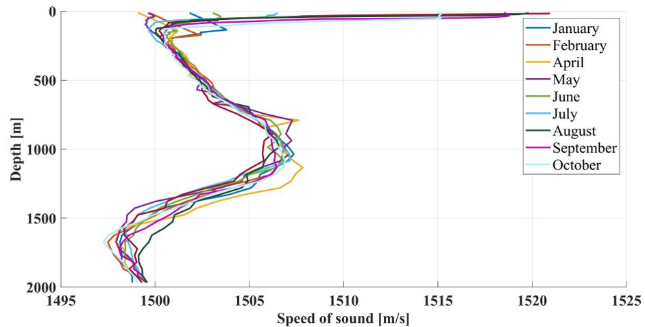
**Figure 2.** Seasonal variation of the speed of sound in column water. The vertical sound speed profile has been considered in the propagation of noise through the sea water. Data of salinity and temperature are missing for March, November, and December.
