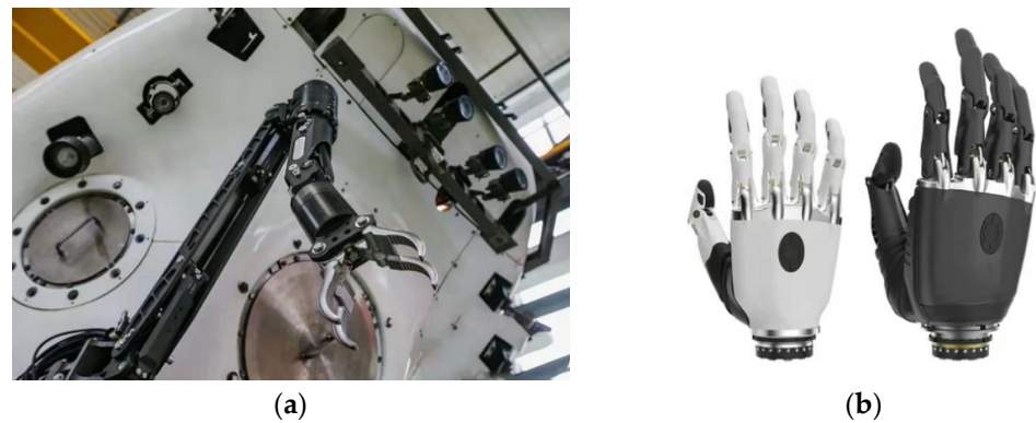
Figure 2. Typical manipulators: (a) Clamp type and (b) Hand type.
