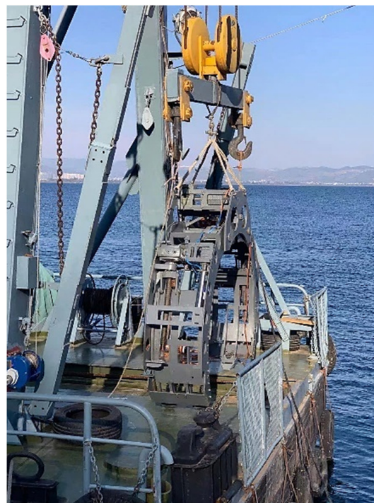
Figure 14. Launch of the manipulator.
