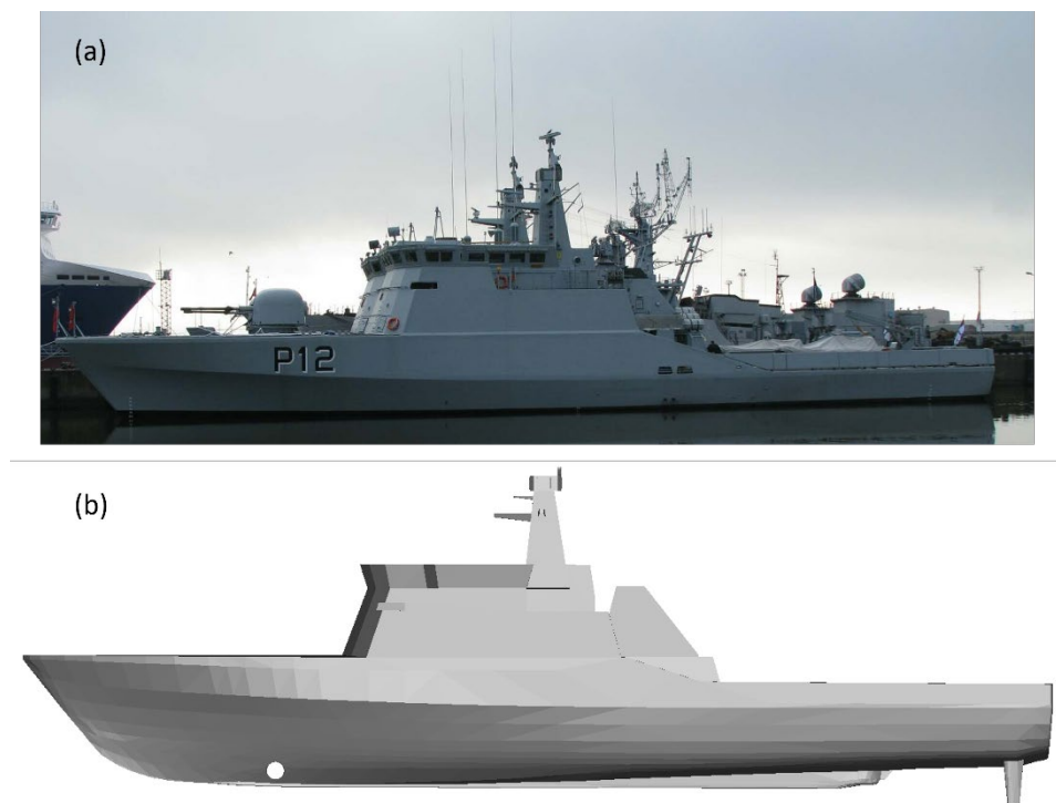
Figure 1. The original (a) and simplified model (b) of the Tejo class vessel.
