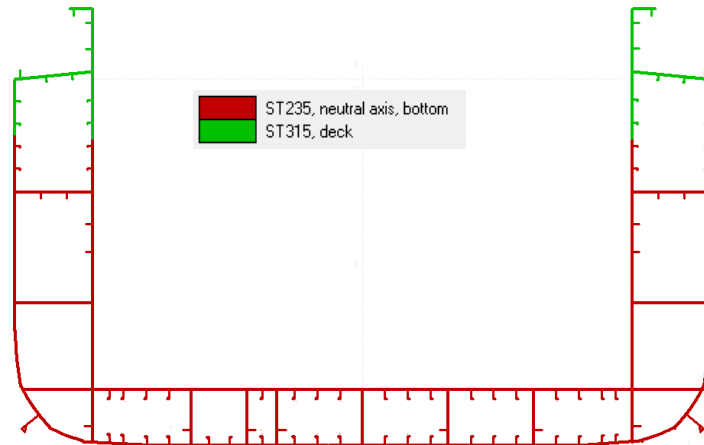
Figure 1. Midship section and material distribution.
