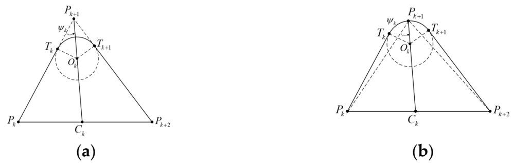
Figure 12. Steering arc connection. (a) Before improvement. (b) After improvement.
