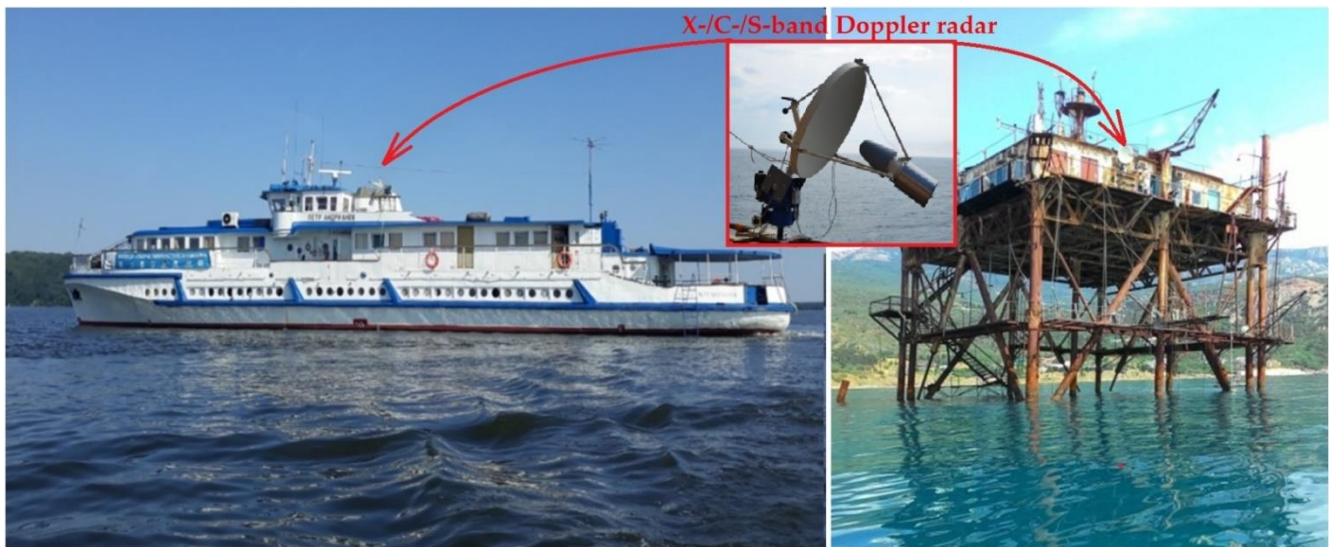
Figure 1. X-/C-/S-band radar mounted onboard the research vessel and the platform.
