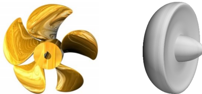
Figure 3. (left) The Potsdam Propeller Test Case (PPTC) without hub. (right) The conformal surface enclosing the propeller and hub. Diameter of the propeller is 250 mm.
