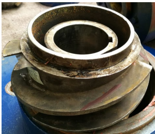
Figure 4. Experimental rig of the multiphase pump. (a) Schematic diagram. (b) Impeller and diffuser.
