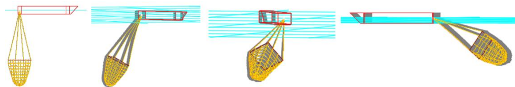
Figure 29. Shape changes of rigid truss trawl in rotating towing under fixed angular velocity at v = 4 m/s.
