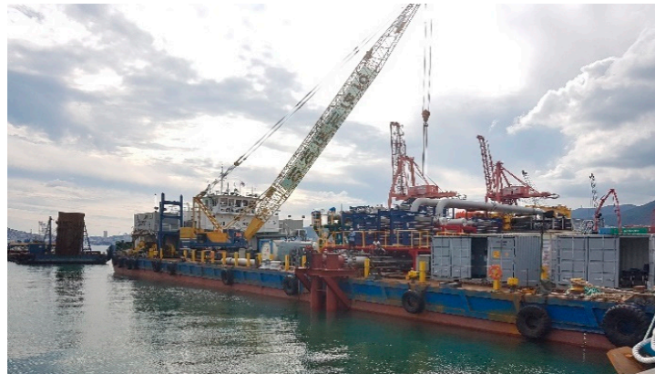
Figure 1. Demonstration of 1 MW floating OTEC in Republic of Korea.
